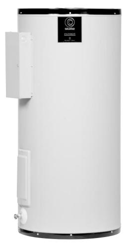
Designed for use as recovery heaters for light-duty hot water supply service. Patriot<sup>™</sup> PCE water heaters are available with tank capacities from 6 through 119 gallons. They can be installed for nonsimultaneous and single element operation (maximum input up to 6 KW), or for simultaneous dual-element operation (maximum input up to 12 KW).
